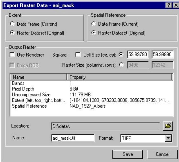
By converting the raster mask image into the GeoTIFF format the mask can be used for the terrain correction of radar images within the MapReady tool.
