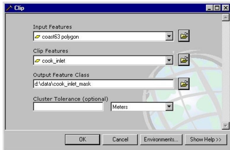
Note that the resulting vector mask inherits the map projection information from the input feature. If you want to use a different projection during the terrain correction process, reproject the input feature into this projection before clipping the area of interest.
